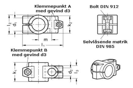
Adjustable clamp lever for d3 = GN 911-M10-55 have to be ordred separately Adjustable clamp lever for d4 = GN 911-M 8-32 have to be ordred separately d1 = 42= 20 d2 = M10d3 = M 8d4 = 65 k1
